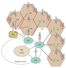
Each mobile communicates via radio with one of the base stations and may be handed-off to any number of base stations throughout the duration of a call.
