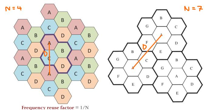
(Each cell within a cluster is only assigned 1/N of the total available channels in the system.)
